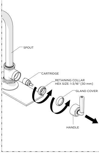
Remove the HANDLE, unthread and remove the GLAND COVER, unthread and remove the RETAINING COLLAR then remove the CARTRIDGE.
