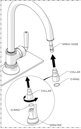
Unthread and remove the COLLAR and O-RING from the top of the SPRAYER then slide the COLLAR and O-RING over the SPRAY HOSE.
