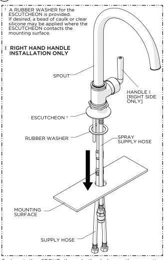
3. Insert the SPOUT through the hole on the mounting surface making sure the RUBBER WASHER provided is beneath the ESCUTCHEON and the HANDLE is aligned on the RIGHT SIDE of the SPOUT.
