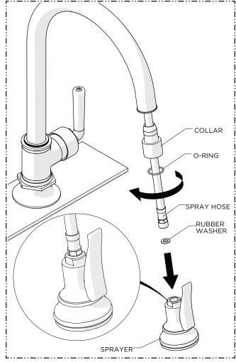
Thread and securely tighten the SPRAY HOSE into the SPRAYER ensuring that the RUBBER WASHER provided is in place.
