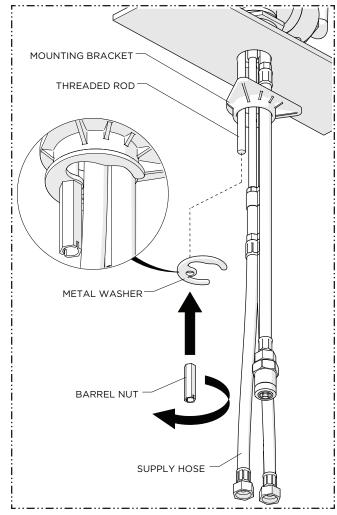
4. Slide the MOUNTING BRACKET over the HOSES and THREADED ROD, place the METAL WASHER onto the THREADED ROD then thread and securely tighten the BARREL NUT onto the THREADED ROD.
