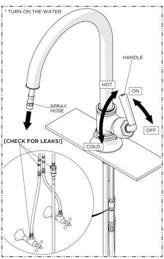
Turn on the water and operate the HANDLE to ensure it functions properly and to flush out any debris in the supply lines then check all connections for leaks and turn off the water.
