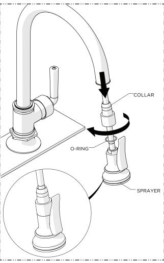
11. Thread and securely tighten the COLLAR back onto the SPRAYER making sure to include the O-RING.
