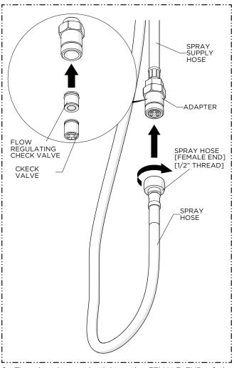
Thread and securely tighten the FEMALE END of the NYLON SPRAY HOSE to the SUPPLY HOSE using the ADAPTER provided.
