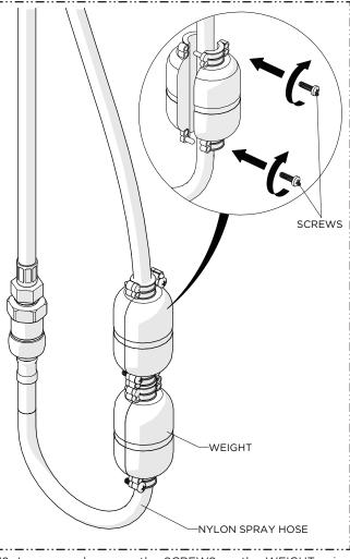
12. Loosen and remove the SCREWS on the WEIGHT using a Phillips head screwdriver, separate the two parts of the WEIGHT, place around the SPRAY HOSE then tighten the SCREWS to secure the WEIGHT in the desired position. Repeat with both WEIGHTS.
