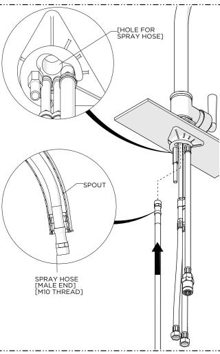
Insert the MALE END of the NYLON SPRAY HOSE through the bottom of the SPOUT until it protrudes from the end of the SPOUT.
