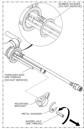
Unthread and remove the BARREL NUT from the THREADED ROD, then remove the METAL WASHER and MOUNTING BRACKET.
