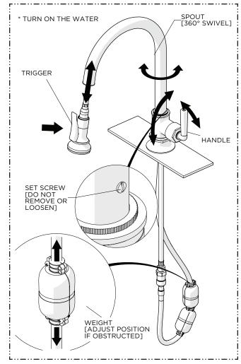
13. Turn on the water and operate the SPRAYER to ensure it functions properly making sure the WEIGHT can move freely beneath the cabinet and the SPOUT is able to swivel properly. Adjust the position of the WEIGHT if necessary.
