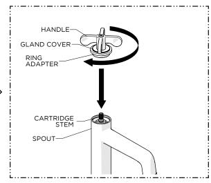
6. With the HANDLE held horizontally thread the RING ADAPTER into the SPOUT until snug.
