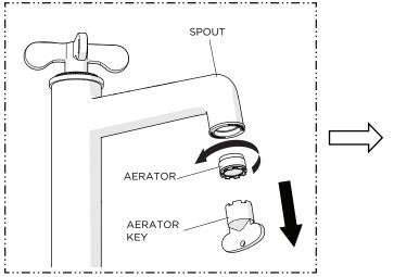
Remove the AERATOR from the SPOUT using the tool provided.
