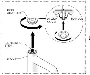
Unthread and remove the RING ADAPTER from the SPOUT, then thread the ADAPTER onto the GLAND COVER until snug.
