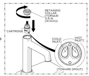
Insert the CARTRIDGE back into the SPOUT as shown then thread and tighten the RETAINING COLLAR to the specified torque settings shown.
