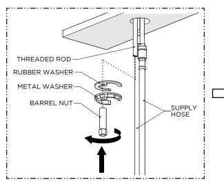
Slide the RUBBER and METAL WASHERS back onto the THREADED ROD then thread and securely tighten the BARREL NUT onto the ROD.
