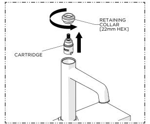
Unthread and remove the RETAINING COLLAR then pull the CARTRIDGE out.
