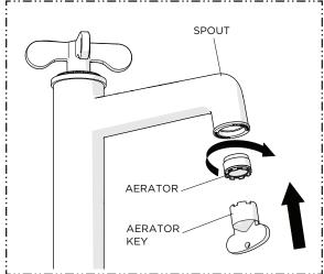
11. Re-install the AERATOR using the tool provided.
