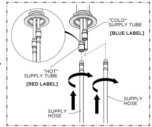
2. Thread and securely tighten the SUPPLY HOSES onto the SUPPLY TUBES on the SPOUT.
